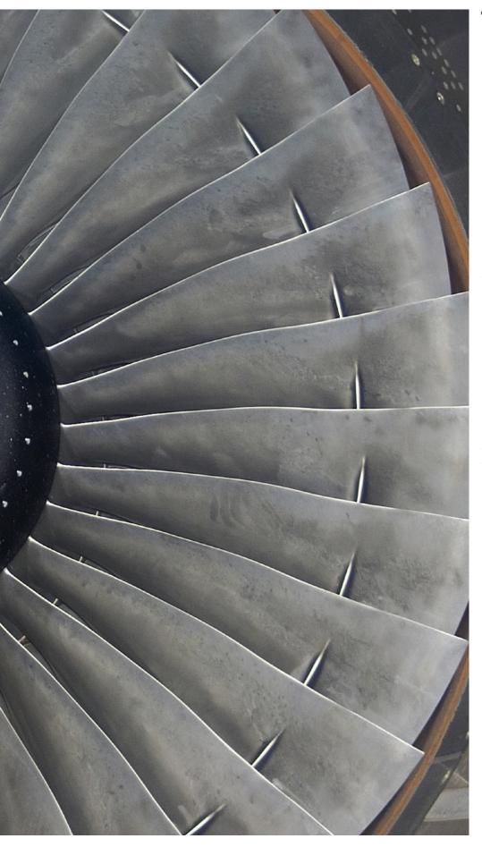
ith the CF6-80E1, General Electric specifically designed an engine for the Airbus A330. The
